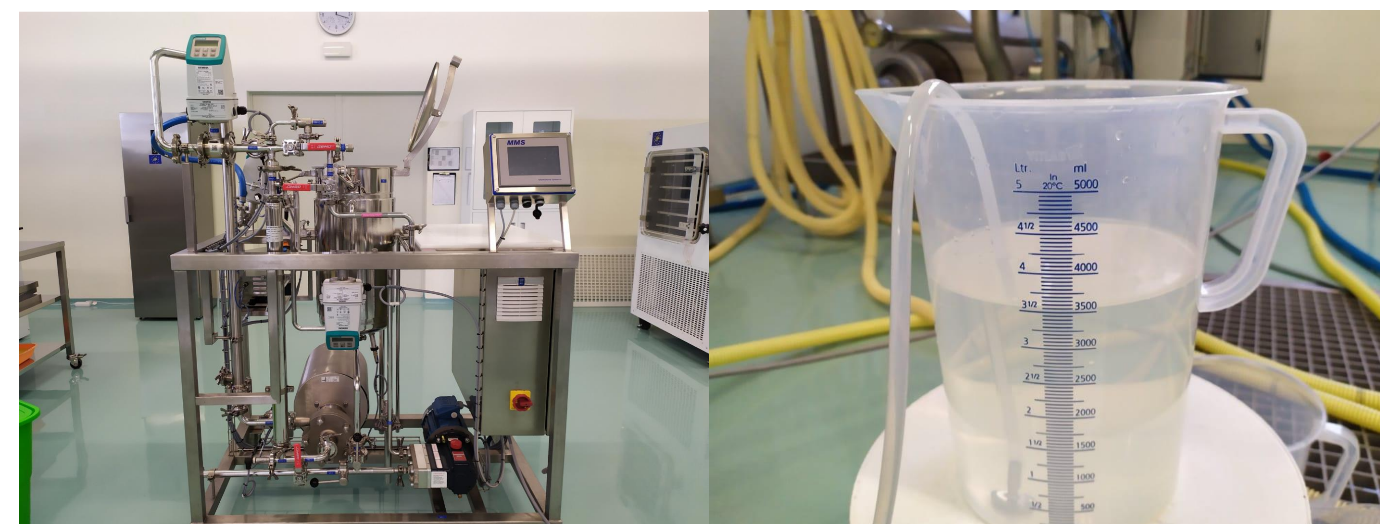
Slika/Figure 1: Naprava MMS SW25 (levo) in permeat prvega poskusa tekem diafiltracije (desno). MMS SW25 filtration device (left) and permeate fraction during diafiltration of the first experiment (right).
